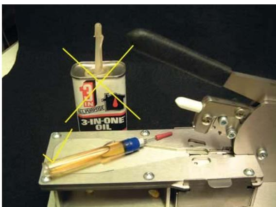
The splitter is supplied with a small oiler pen that contains a suitable lubricant. DO NOT USE LIGHT MULTI-PURPOSE LUBRICANT. Any multi-grade engine oil or gearbox oil can be used. These oils contain additives that will resist high pressures (surface stresses) and will protect key features against wear, HOUSEHOLD OILS WILL NOT!
