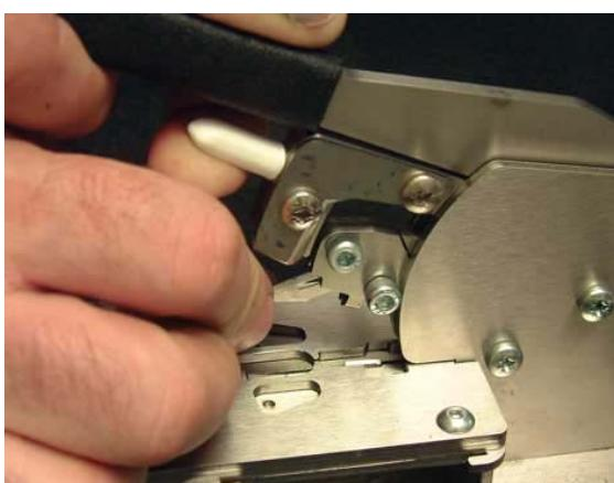
Loosen the two clamp screws by about 1/3 of a turn each.
