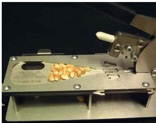
Provision to clear any residual test grains has been made. One of the sample trays can act as a collector tray.
